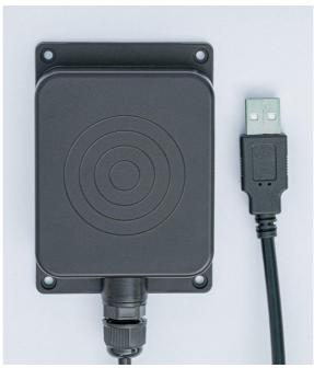
EC-RF615 is the EC-LINK company launched a UHF RFID antenna integrated card reading module, integrated 915Mhz card reading module and ceramic antenna, the product uses the industry general USB connector, a cable to achieve power supply and data transmission, can be easily installed in size-limited applications.
