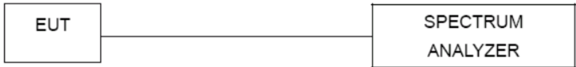
Figure 67. Conducted Output Power Bench measurement
