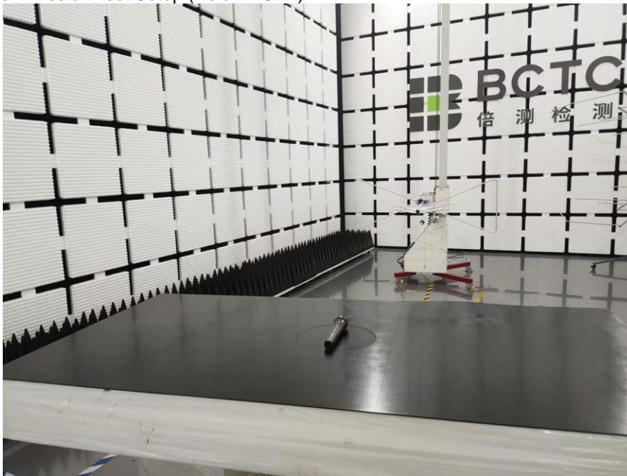
Spurious Emission Test Setup (Below 1GHz)
