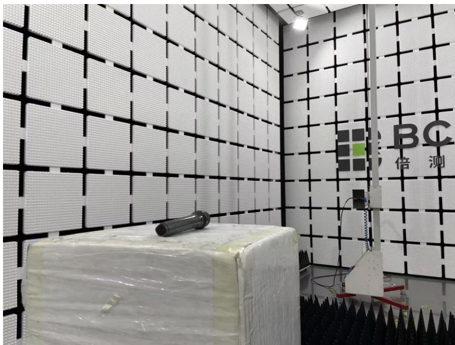
Spurious Emission Test Setup (Above 1GHz)
