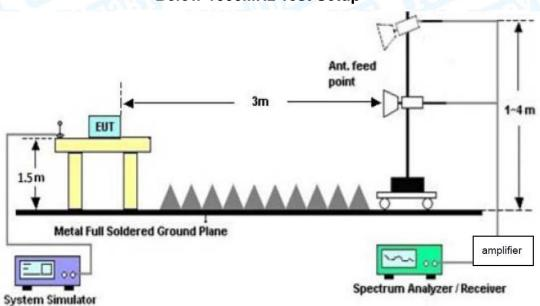
**Above 1GHz Test Setup**
