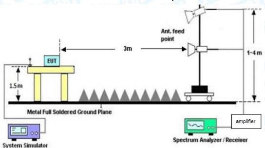
**Above 1GHz Test Setup**
