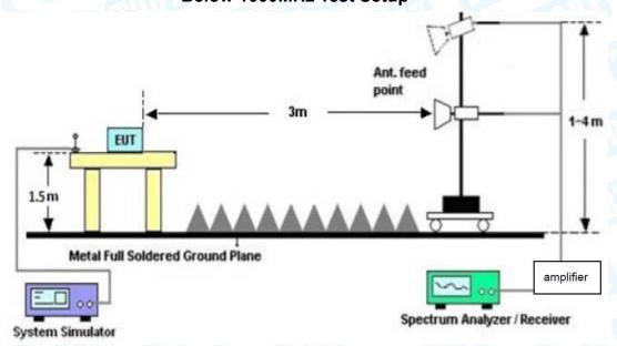
**Above 1GHz Test Setup**
