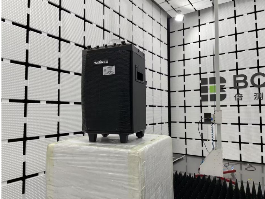
Spurious Emission Test Setup (Above 1GHz)
