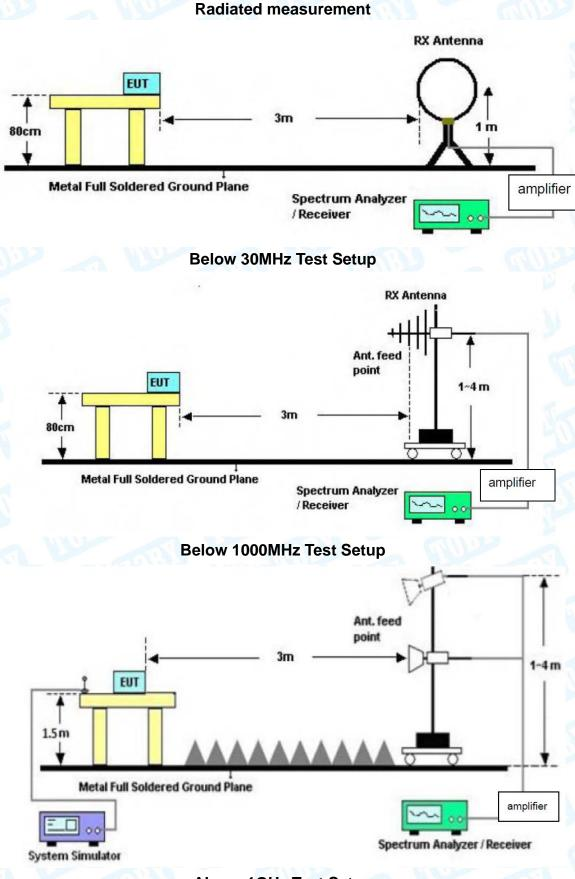
Above 1GHz Test Setup
