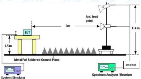
**Above 1GHz Test Setup**
