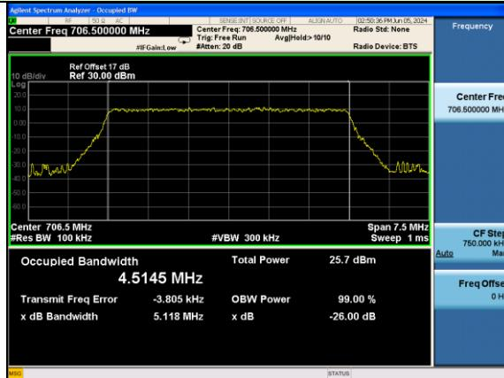
Test Mode: LTE Band 17 / 5MHz /16-QAM
