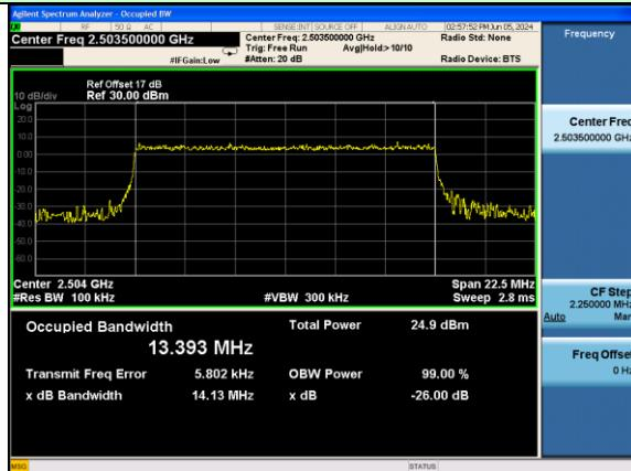
Test Mode: LTE Band 41 / 15MHz /16-QAM
