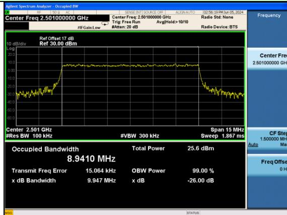
Test Mode: LTE Band 41 / 10MHz /16-QAM
