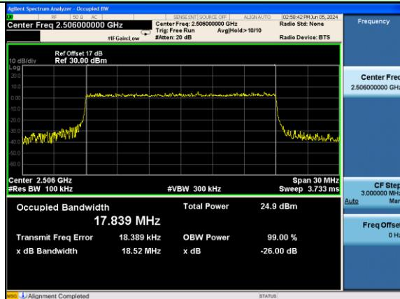
Test Mode: LTE Band 41 / 20MHz /16-QAM
