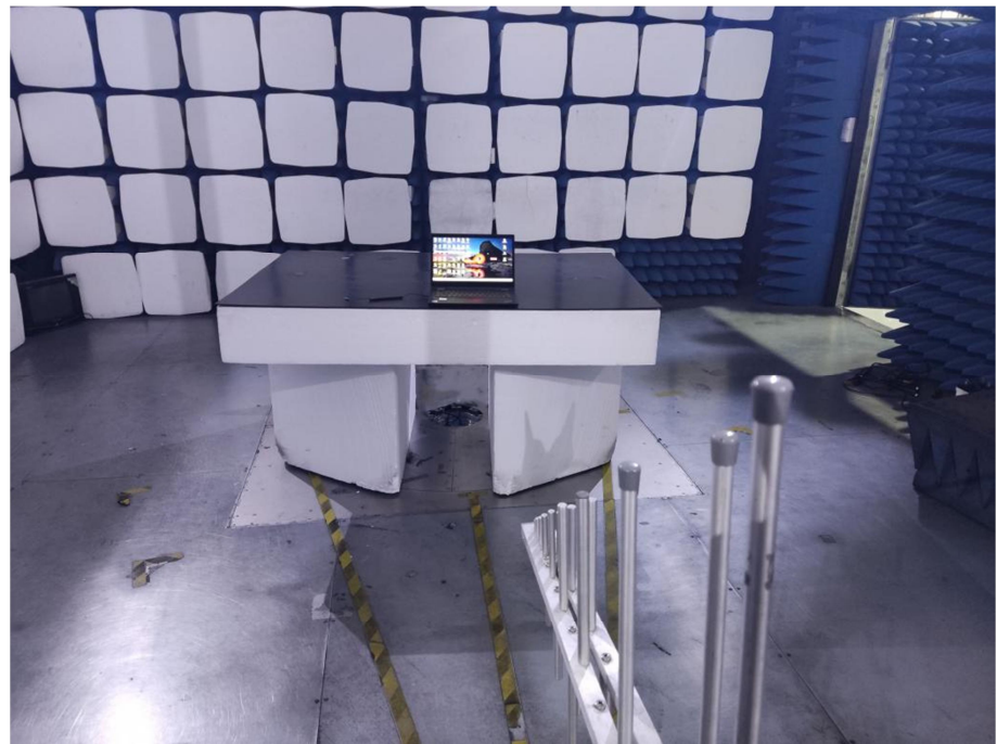
Radiation Emission Test Setup (30MHz to 1GHz)
