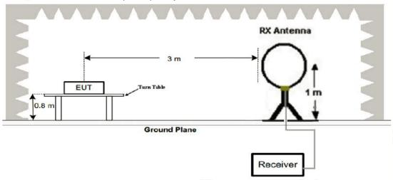
2. Radiated Emission Test-Up Frequency 30MHz~1GHz
