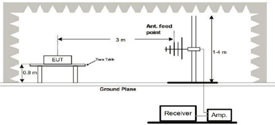
3. Radiated Emission Test-Up Frequency Above 1GHz
