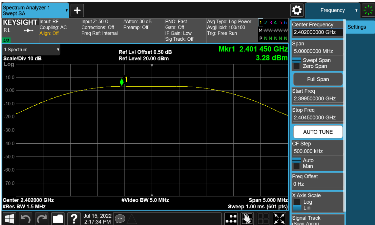
Figure 4: Peak Output Power, BLE_2Mbps_2402MHz
