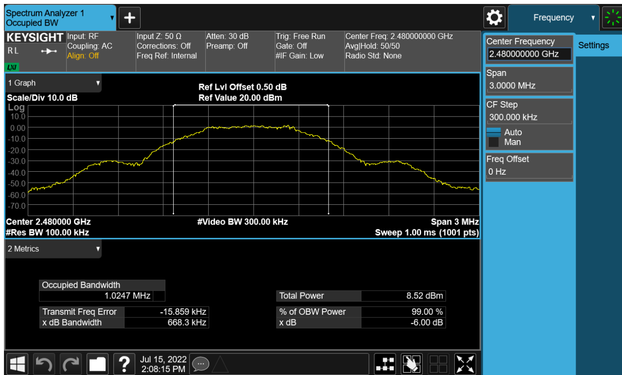
Figure 10: 6dB Bandwidth, BLE_2Mbps_2402MHz
