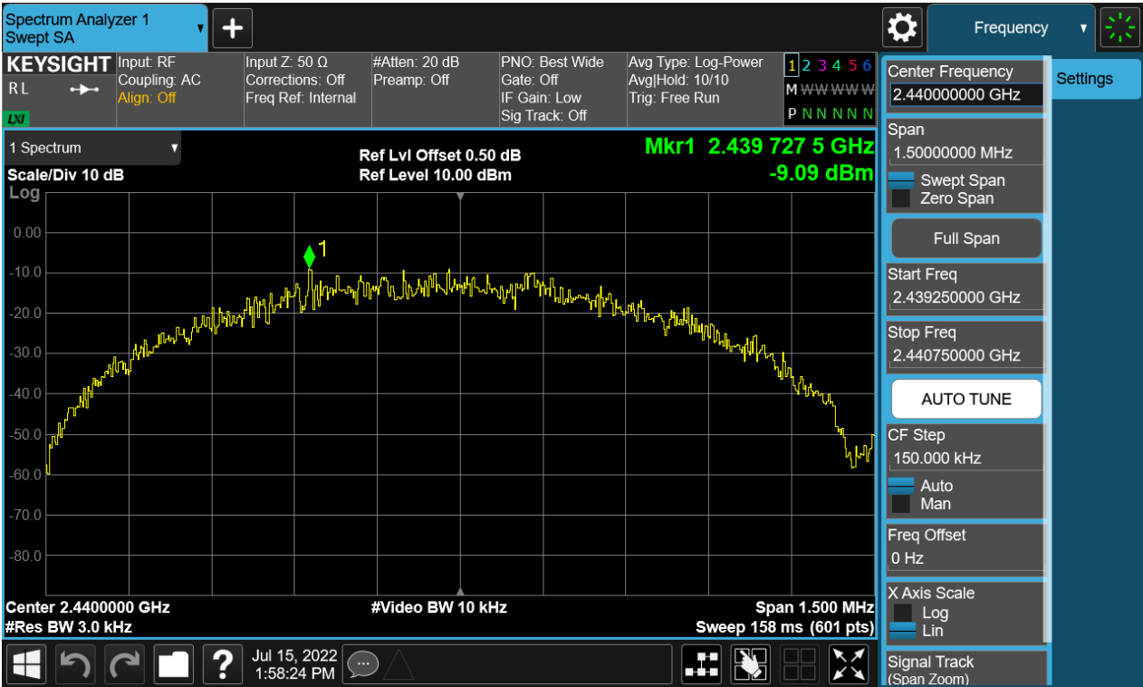
Figure 14: Power Spectral Density, BLE_1Mbps_2440MHz
