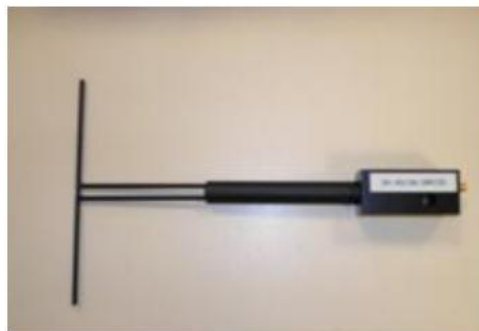
Figure 1 – Satimo COMOSAR Validation Dipole
