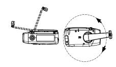
For subsequent charges, turn the handle crank for 2-3 minute(crank speed>=130rmp) to produce: 10~15 minutes of continuous light for three LED; 10-15 minutes of continuous radio usage (medium volume); 3-5 minutes of talk time.
