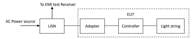
Note: for detail, please refer to the test setup photo for each test item
