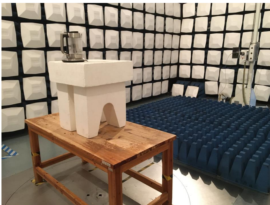
Test Setup For Radiated Emission (Above 1GHz)
