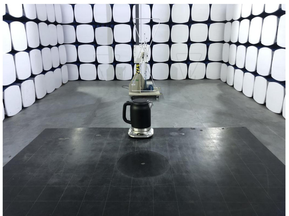
Radiation Emission Test Setup (30MHz to 1GHz)
