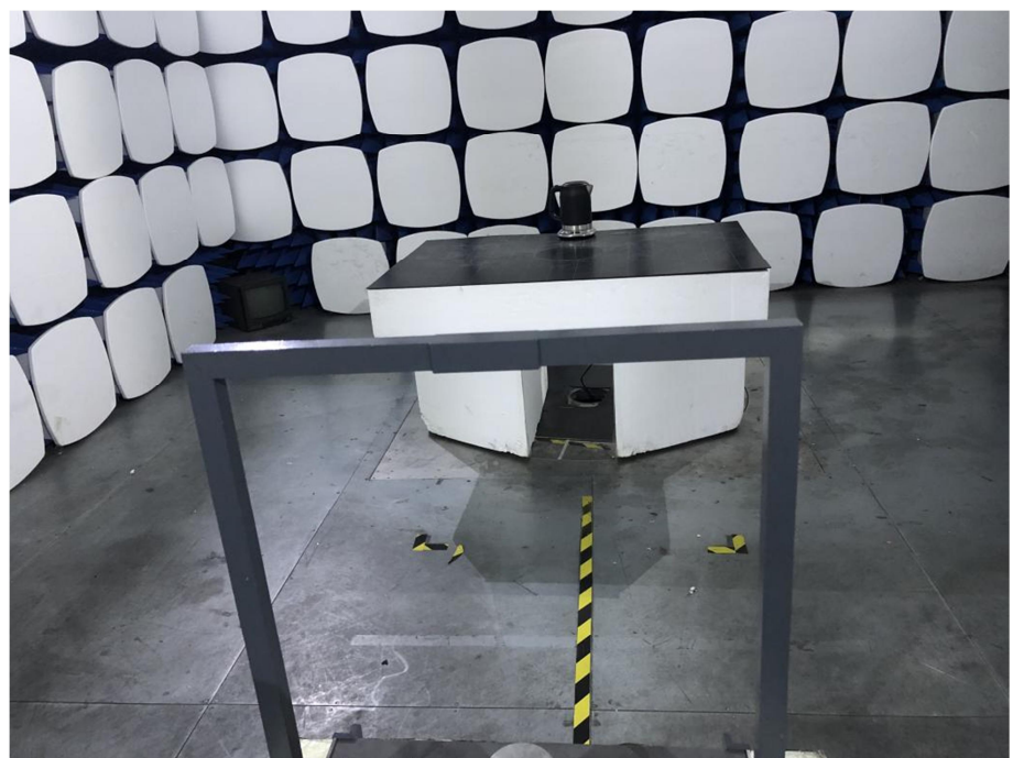
Radiation Emission Test Setup (Below 30MHz)
