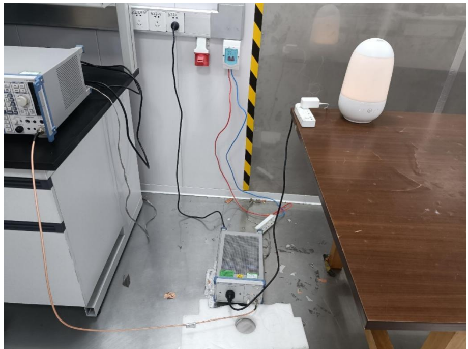
Conducted Emission Test Setup
