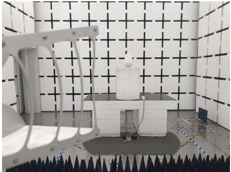
Radiation Emission Test Setup (1GHz to 18GHz)
