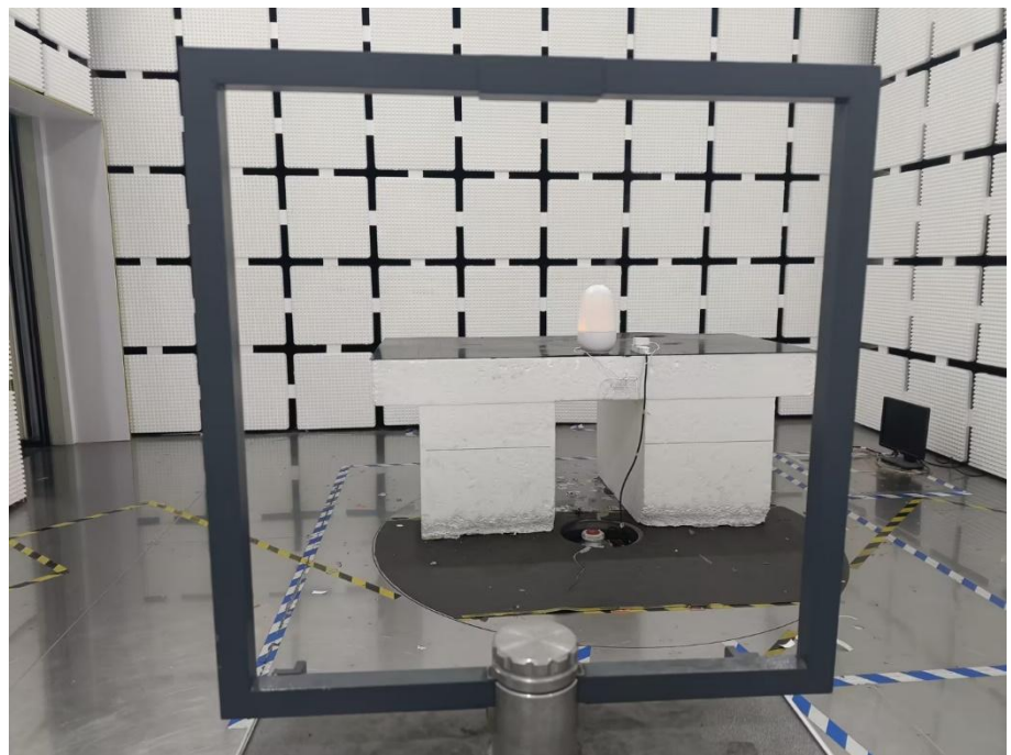
Radiation Emission Test Setup (Below 30MHz)
