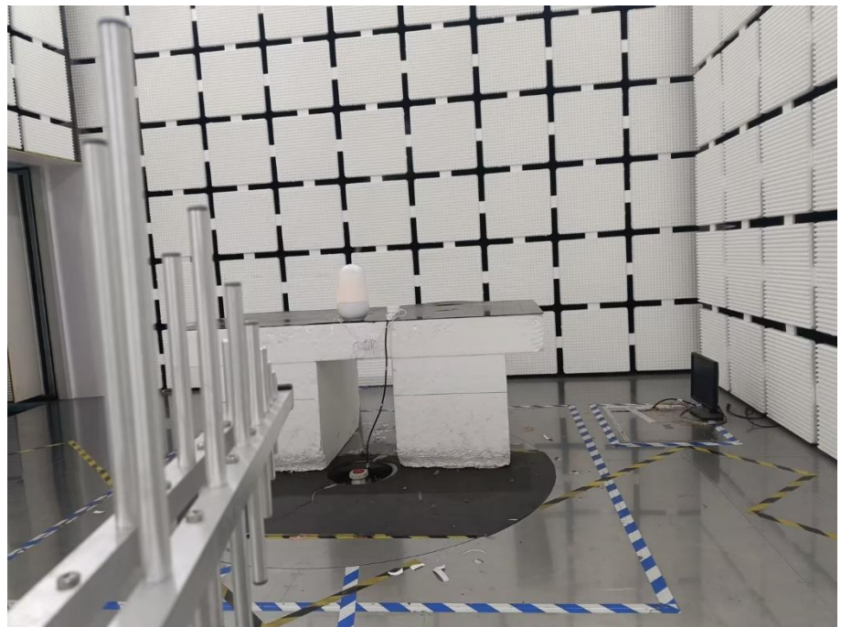
Radiation Emission Test Setup (30MHz to 1GHz)
