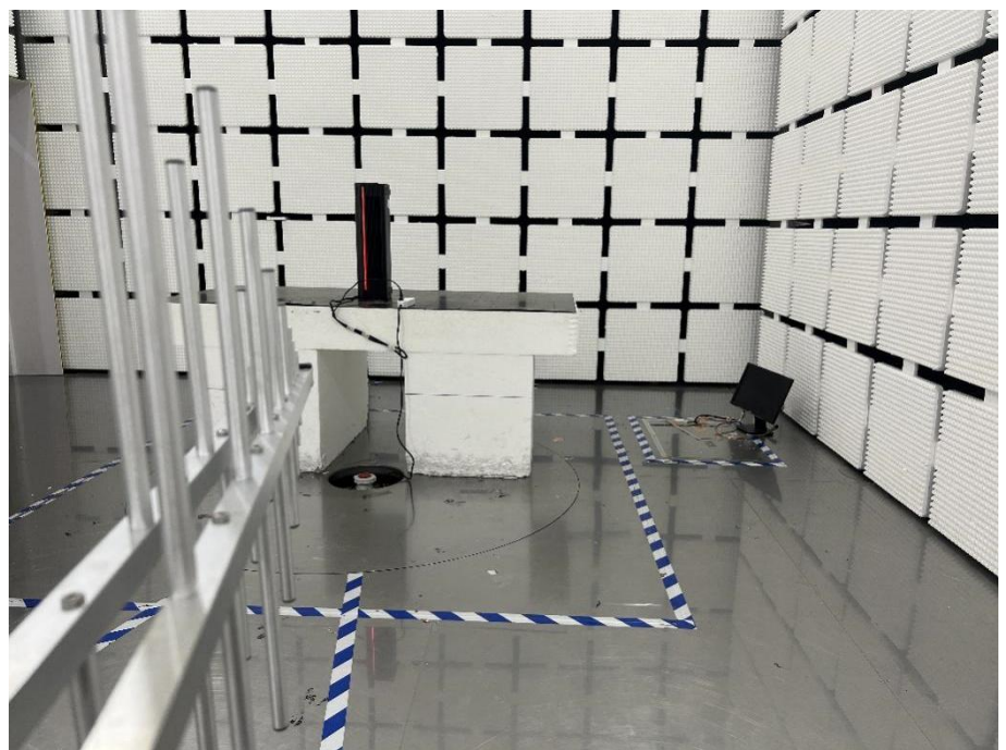
Radiation Emission Test Setup (30MHz to 1GHz)
