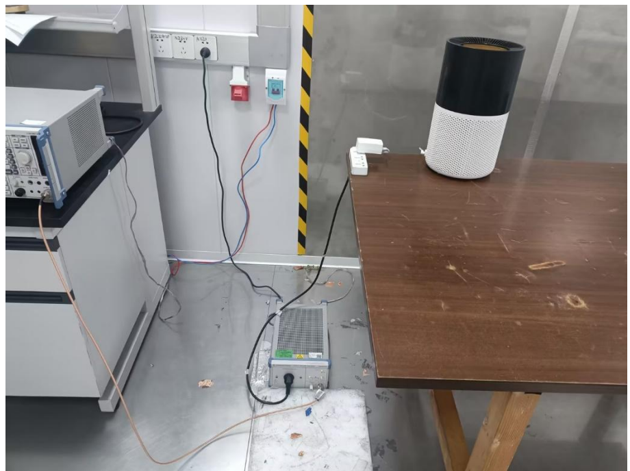
Conducted Emission Test Setup
