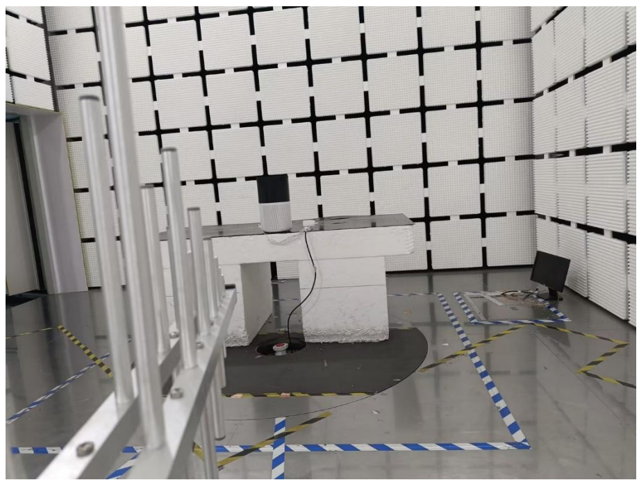
Radiation Emission Test Setup (30MHz to 1GHz)
