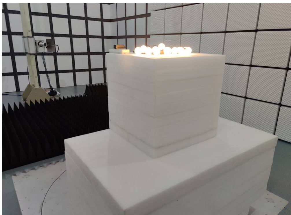
Photo of Radiated Emission Measurement (Above 1G)
