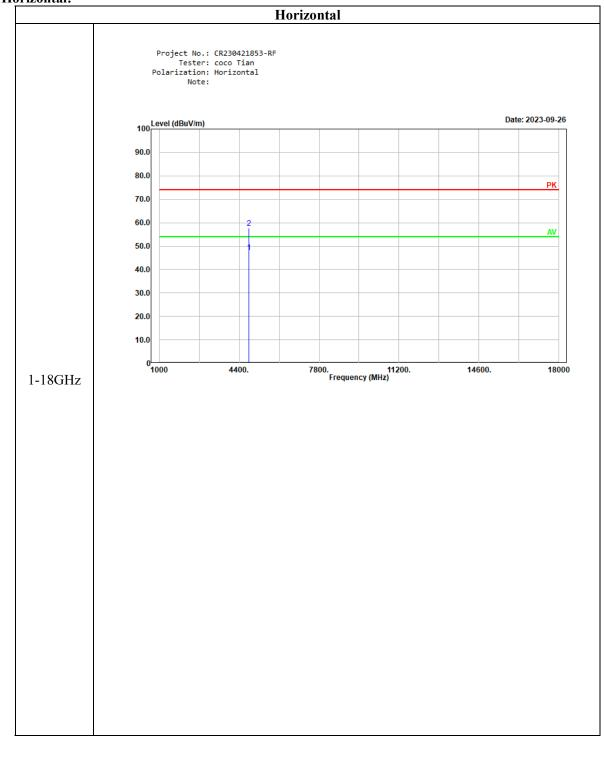
Listed with the worst harmonic margin test plot (BLE 1Mbps low channel) Horizontal:
