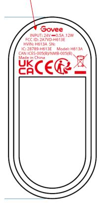
The label shown shall be permanently affixed at a conspicuous location on the device and be readily visible to the user at the time purchase (Labeling requirements per 2.925)
