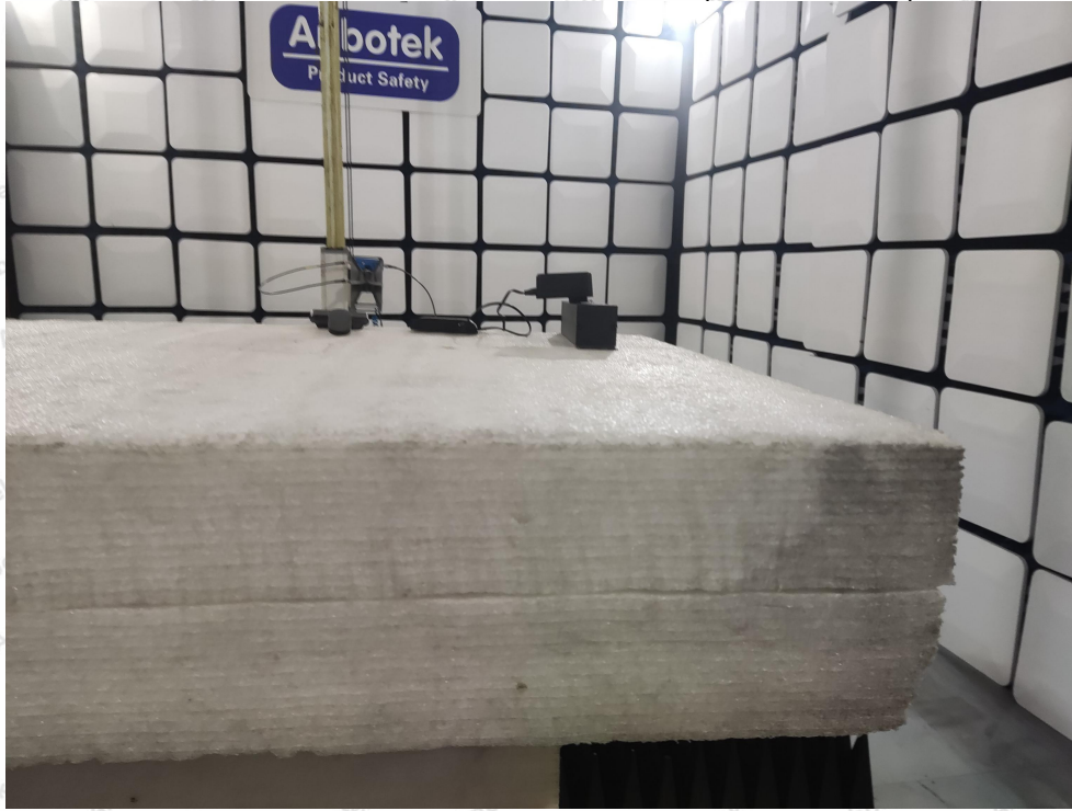
Photo of Radiation Emission Test (above 1GHz)
