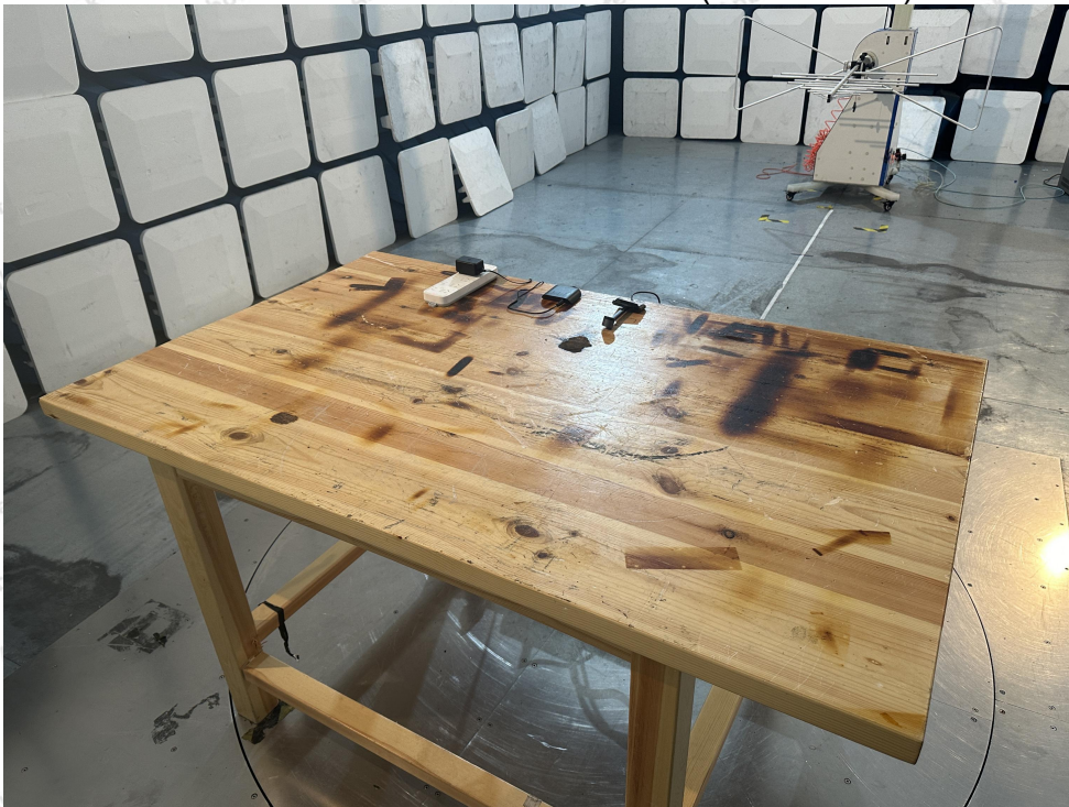
Photo of Radiation Emission Test (below 1GHz)
