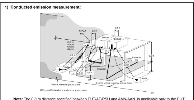
**Note:** The 0.8 m distance specified between EUT/AE/PSU and AMN/AAN, is applicable only to the EUT being measured. If the device is AE then it shall be >0.8 m.
