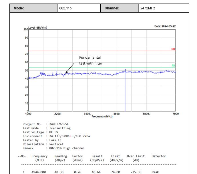
Remarks: Factor = Antenna factor + Cable loss - Preamp gain Result = Reading + Factor Over Limit = Result - Limit
