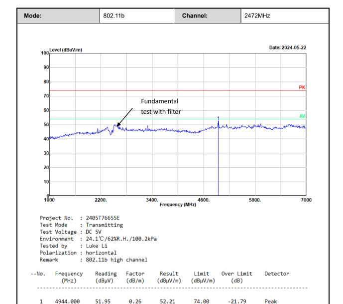
Remarks: Factor = Antenna factor + Cable loss - Preamp gain Result = Reading + Factor
