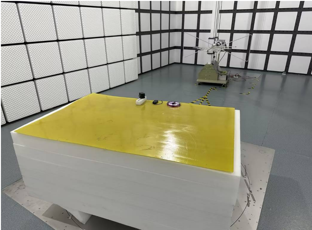
Photo of Radiated Emission Measurement (Above 1G)
