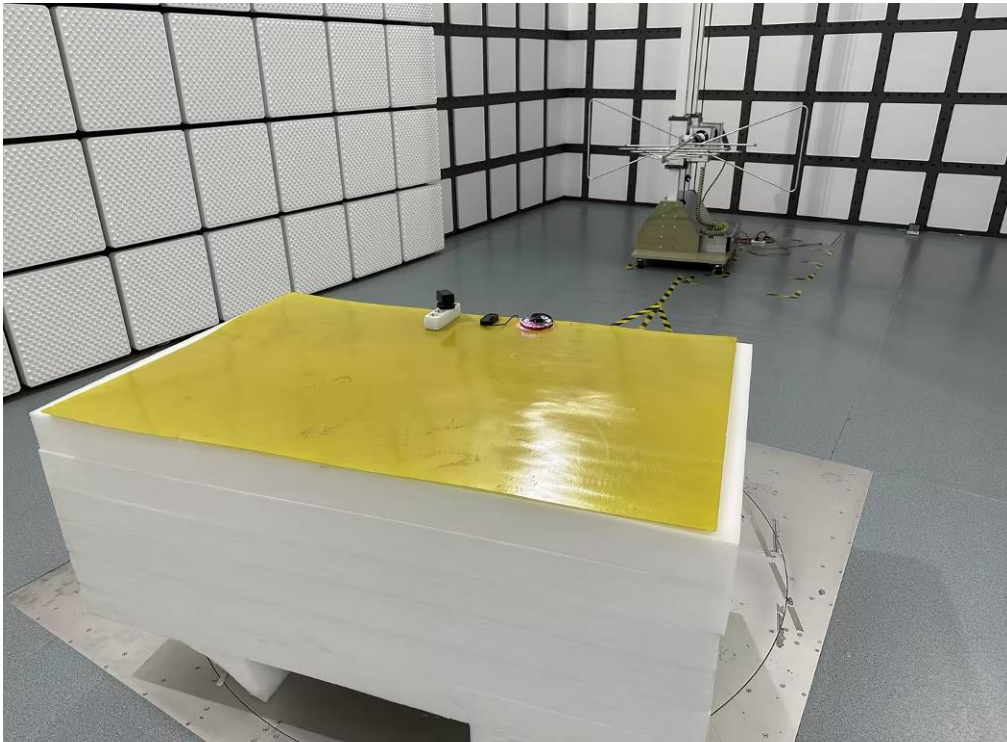
Photo of Radiated Emission Measurement (Above 1G)
