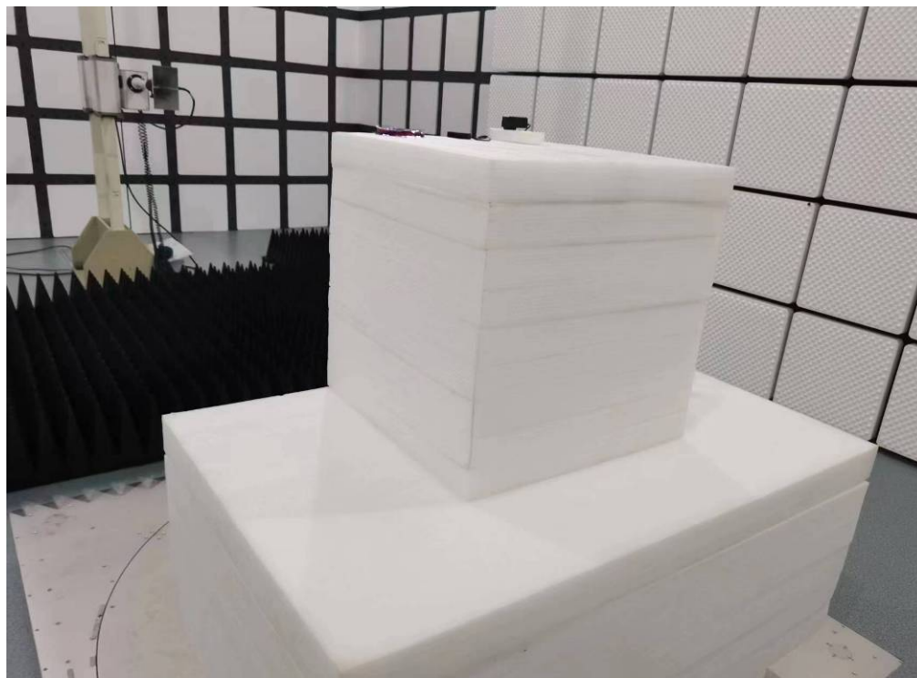
Photo of Radiated Emission Measurement (Above 1G)
