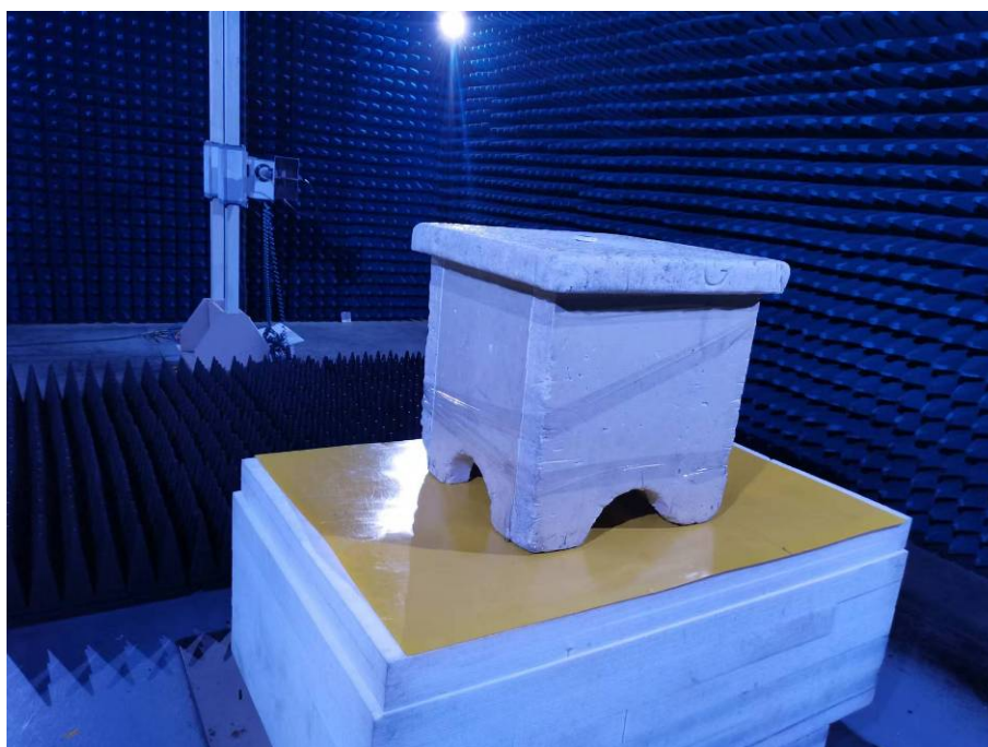
Photo of Radiated Emission Measurement (Above 1G)
