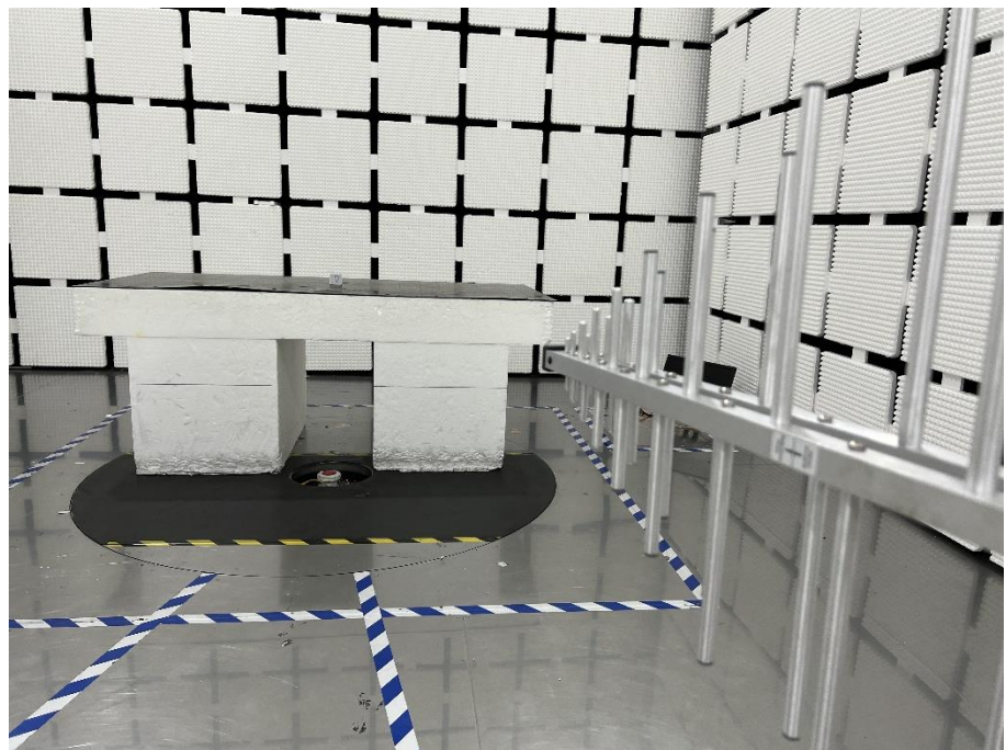
Radiation Emission Test Setup (30MHz to 1GHz)
