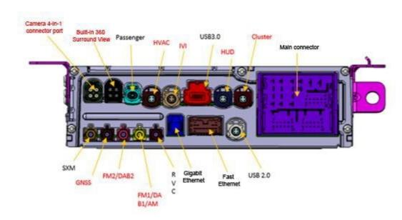
Camera 4-in-1 connector port: It can connect up to four 2-megapixel cameras for inputting video data from DVR, DMS, and OMS cameras.
