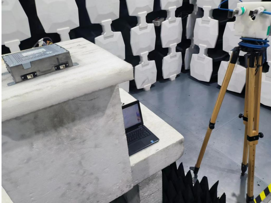
Description: Radiated Emission Test Setup (Above 18GHz)
