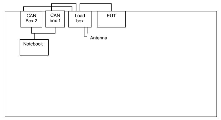
The EUT is power by battery, the load box is used to simulate the EUT working status, and the antenna is though the load box connects to the EUT.
