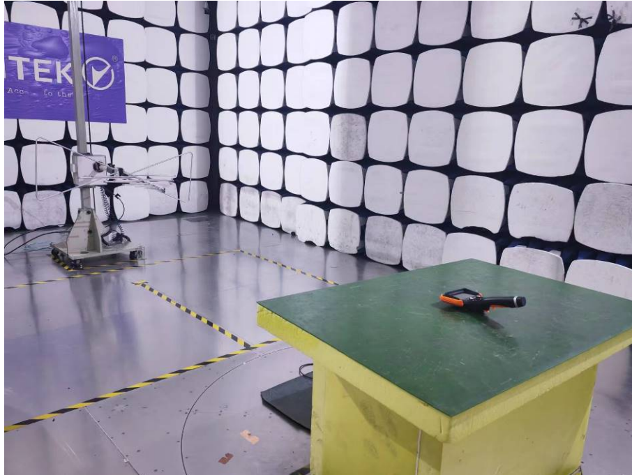
Spurious Emission Test Setup (Above 1GHz)
