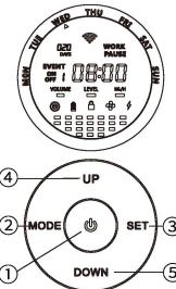
Press MODE 5 seconds to reset the machine and WIFI model. Press Set 5 seconds to lock all keypads, then Press Set 5 seconds again to unlock. Press on/off to pause or start the atomization. Press the on/off 5 seconds to turn on/off the oil level light.
