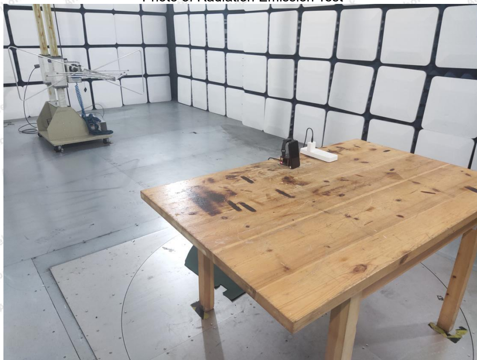
Photo of Radiation Emission Test
