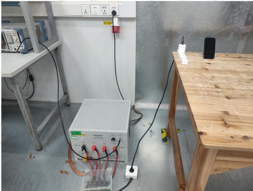
Photo of Conducted Emission Measurement
