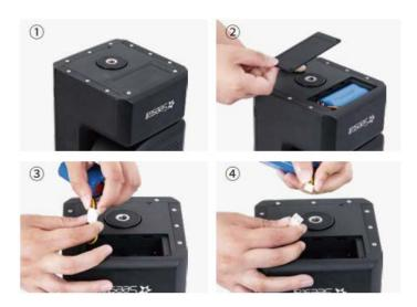
1. Note: Before replacing or removing the battery, make sure the device is turned off and disconnected from the power source. Additionally, handle the process with care to avoid damaging the device or battery.
