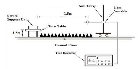
The radiated emission tests were performed in the 3 meters chamber test site, using the setup accordance with the ANSI C63.10-2013. The specification used was FCC 15.209, FCC 15.407, RSS-247, RSS-Gen limits.
