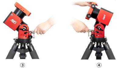
Manipulate the equatorial mount to slide and adjust the "altitude fine-tuning knob," allowing the hex screw to slide to the bottom end of the hole's slide rail, with the scale screw indicating at the 90° position. At the same time, expose the hex screw and retighten the hex screws on both sides (Note: After adjusting the gear position, be sure to tighten the gear screws firmly, otherwise the equipment may become loose and the gear adjustment function can be easily damaged).
