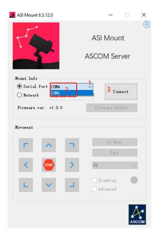
\* Note: The port number to select can be found in Computer Management, as shown below; alternatively, you can try each of the serial ports provided in the ASI Mount ASCOM interface one by one.
