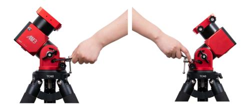
Pull the mount head, you' Il notice the two hex screws are sliding to the bottom place of the inner slideway, while the latitude scale is currently pointing at 45°. Retighten the hex screws on both sides.
