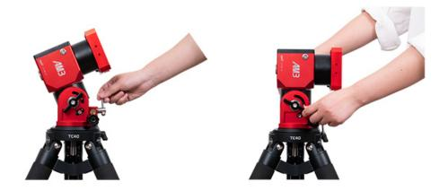
To switch from Gear two to Gear one, just take the above steps in reverse.
