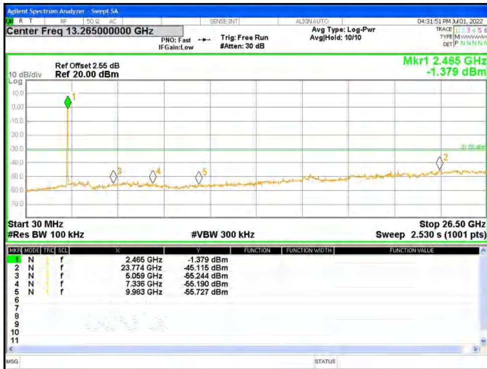
Tx. Spurious NVNT n40 2422MHz Ant1 Ref
