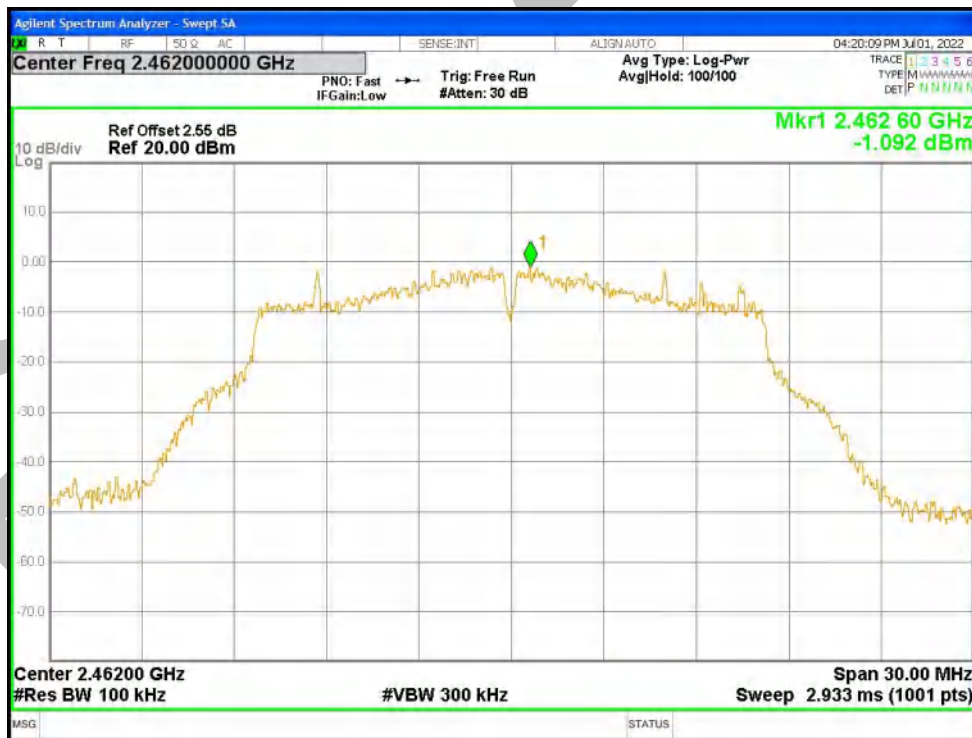
Band Edge NVNT g 2462MHz Ant1 Emission
