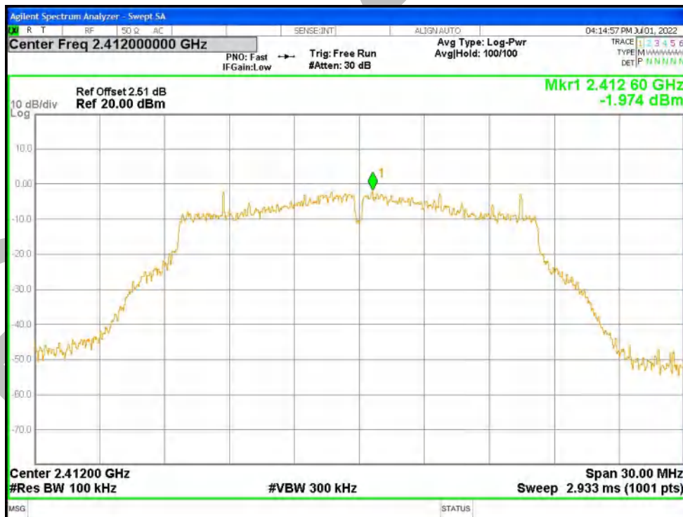
Tx. Spurious NVNT g 2412MHz Ant1 Emission
