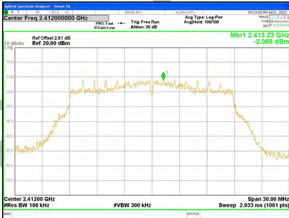
Tx. Spurious NVNT n20 2412MHz Ant1 Emission
