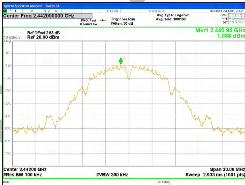
Tx. Spurious NVNT b 2442MHz Ant1 Emission
