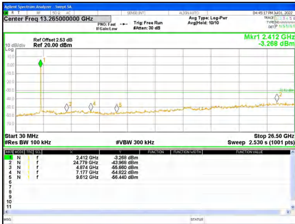
Tx. Spurious NVNT n40 2452MHz Ant1 Ref
