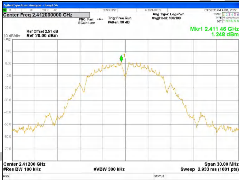
Band Edge NVNT b 2412MHz Ant1 Emission
