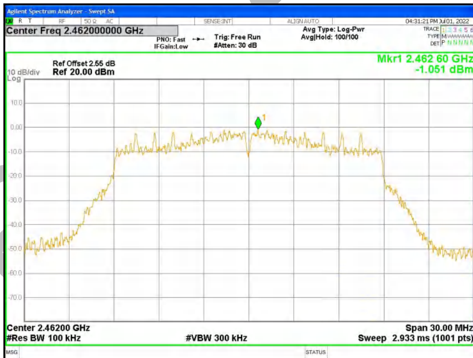
Tx. Spurious NVNT n20 2462MHz Ant1 Emission
