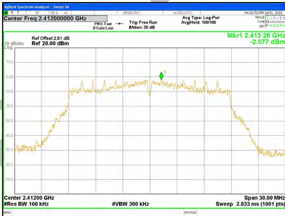
Band Edge NVNT n20 2412MHz Ant1 Emission
