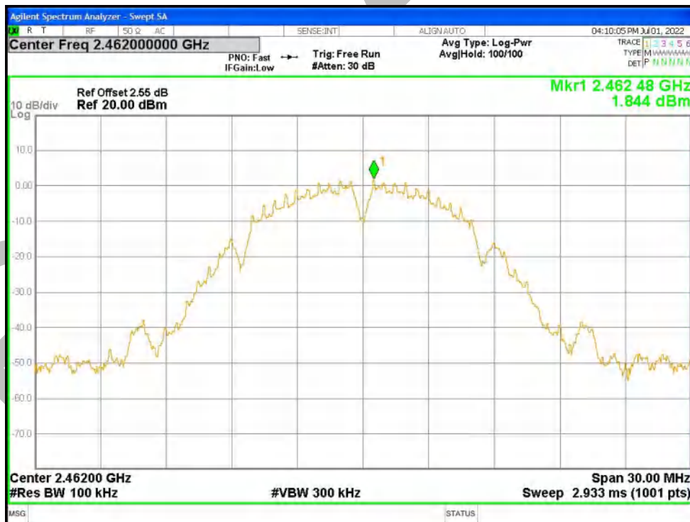
Band Edge NVNT b 2462MHz Ant1 Emission
