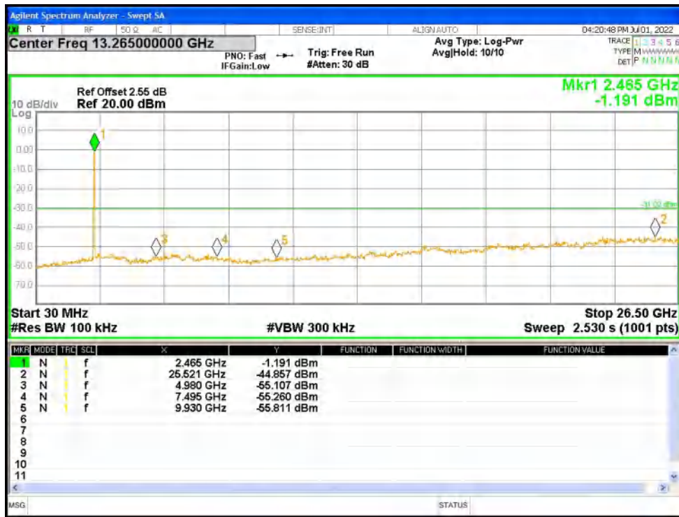
Tx. Spurious NVNT n20 2412MHz Ant1 Ref
