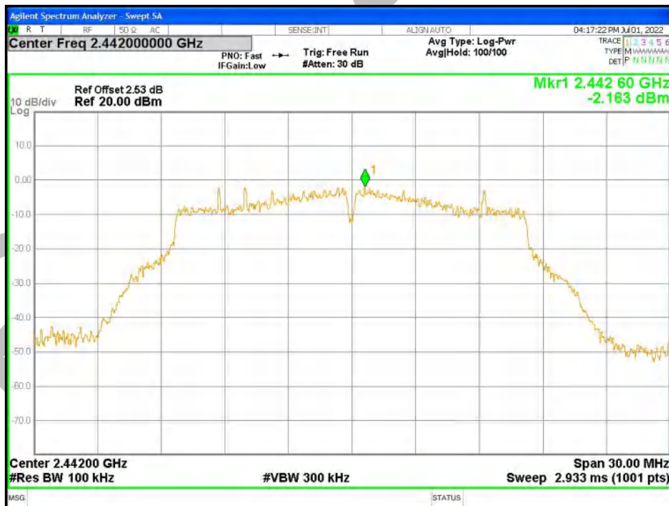
Tx. Spurious NVNT g 2442MHz Ant1 Emission
