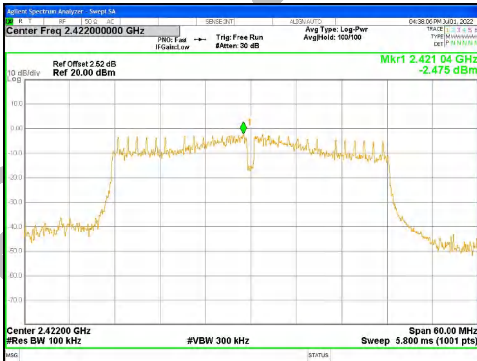
Tx. Spurious NVNT n40 2422MHz Ant1 Emission
