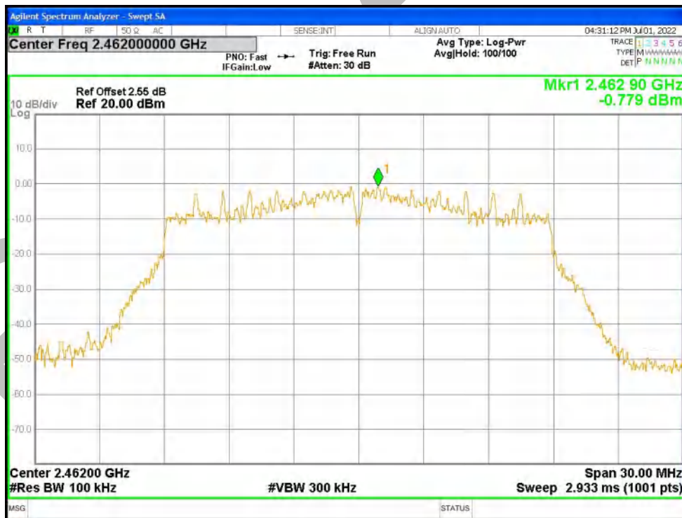
Band Edge NVNT n20 2462MHz Ant1 Emission
