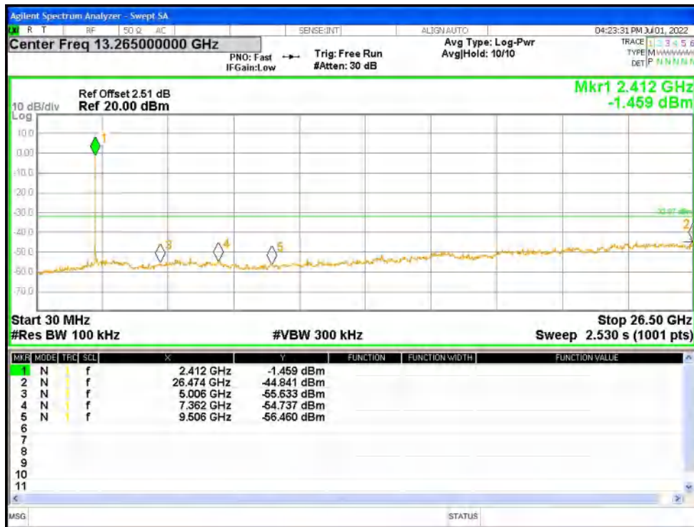
Tx. Spurious NVNT n20 2442MHz Ant1 Ref
