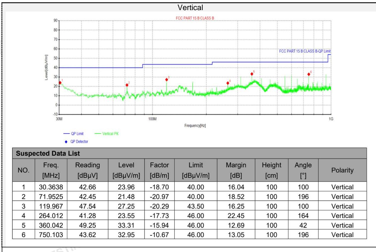
Note:1).Level (dB $\mu$ V/m)= Reading (dB $\mu$ V)+ Factor (dB/m)
