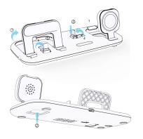
There are 2 ways to open the contact port of the watch: ①Push the contact port upwards to stand up or ②Push it up from the back with your finger
