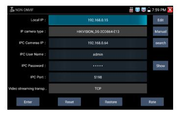
**Local IP**: This is the tester's IP address. Click "Edit" to enter "IP setting" and change the tester's IP address settings.
