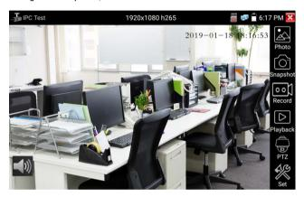
If IP address setting has error or IP camera is not connected.. The tester prompts "Network Frror"
