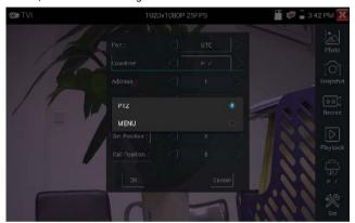
Input calling dome camera menu address code, after finishing the parameter settings, you can press the yey or clique icon to call the dome camera menu.
