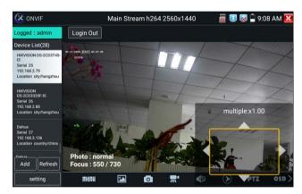
When the image is enlarged, if not operate on touch screen, it can operate by the keyboard, presenthe key to zoom in, presenthe key to zoom out, press upward and downward key to move image.
