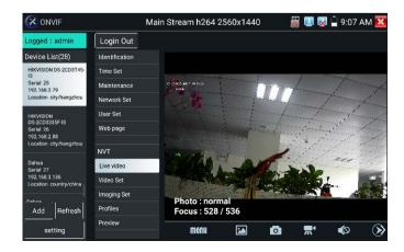
**ONVIF PTZ control:** Tap the image in the direction you want the PTZ camera to move. Tap the left side of the image to move left, right to go right, up to go up and down to go down.
