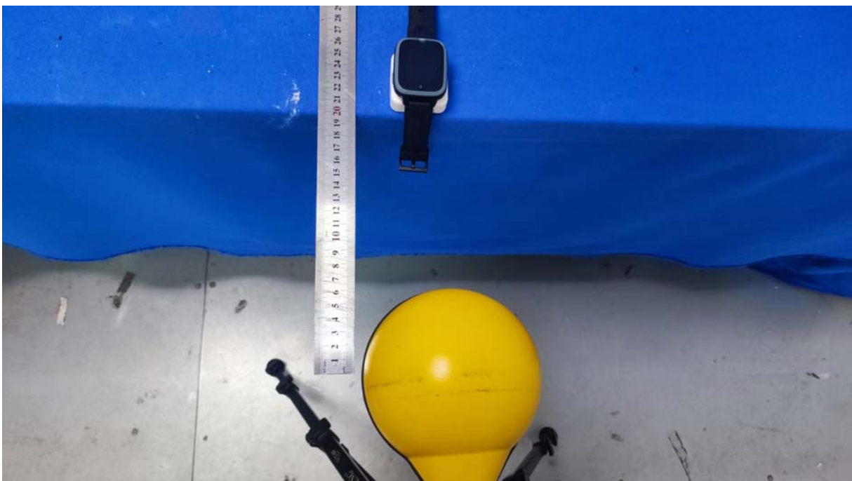
Test Position B-20cm from the edge of EUT to the geometric center of the probe
