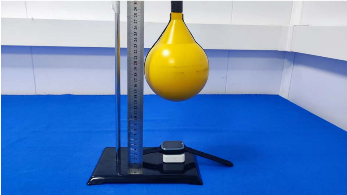
Test Position E-20cm from the edge of EUT to the geometric center of the probe
