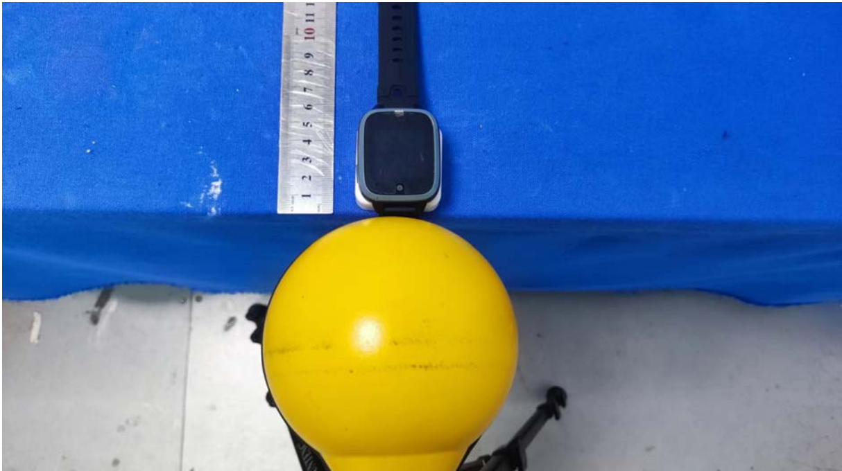
Test Position B-0cm from the edge of EUT to the geometric center of the probe
