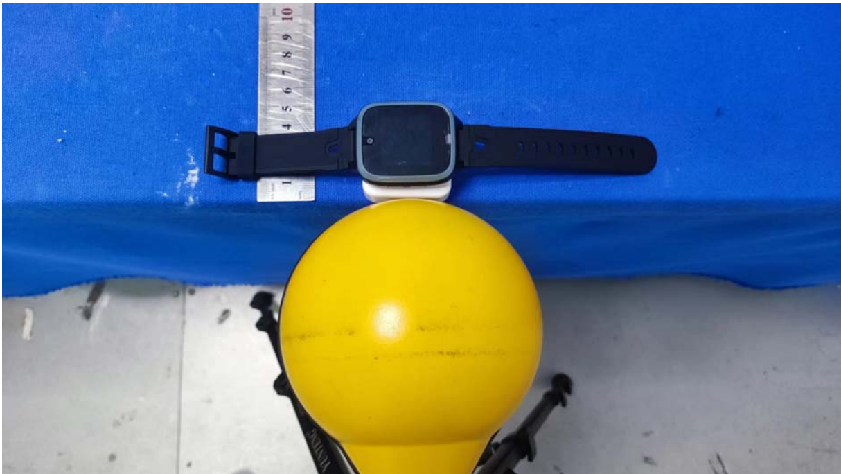
Test Position C-0cm from the edge of EUT to the geometric center of the probe
