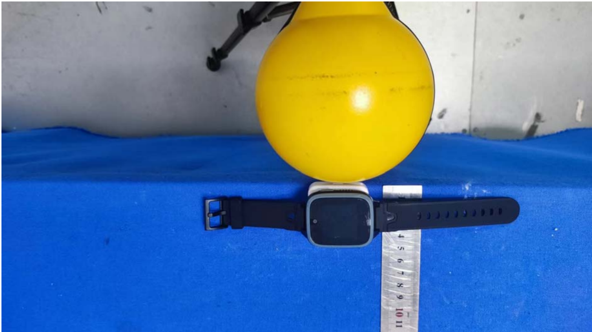
Test Position A-0cm from the edge of EUT to the geometric center of the probe
