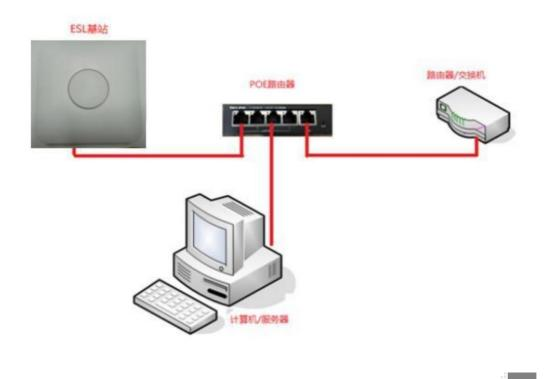
(ESL Base Station Configuration Network Diagram)
