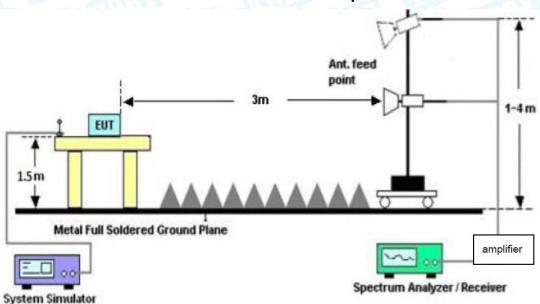
**Above 1GHz Test Setup**
