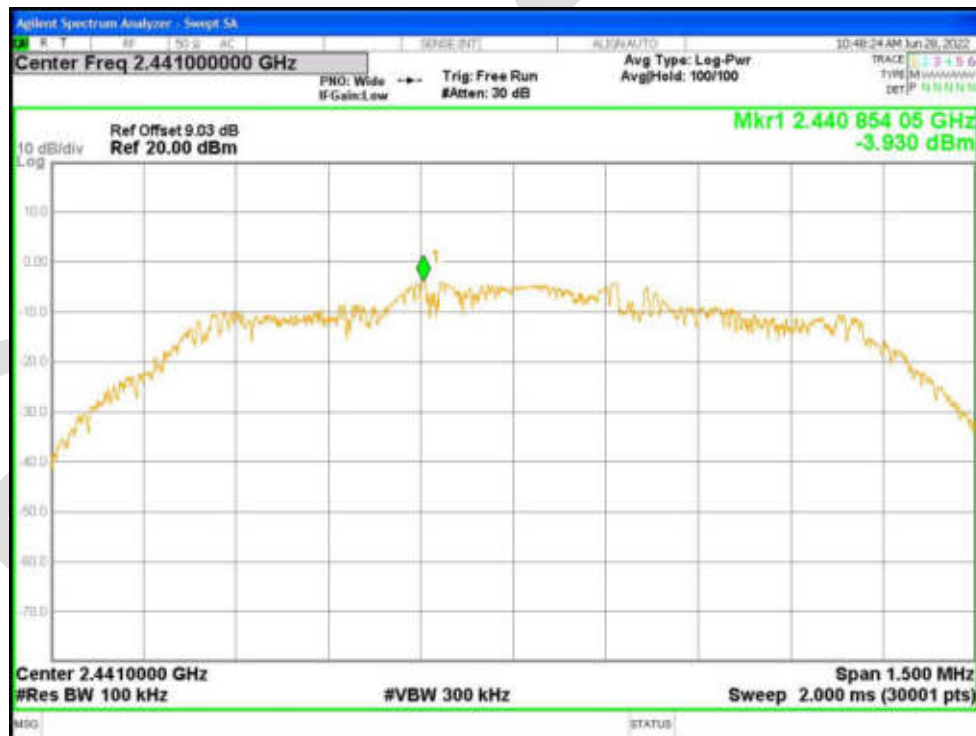
Tx. Spurious NVNT 3-DH1 2441MHz Ant1 Emission
