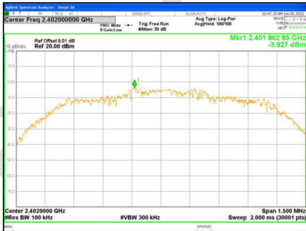
Tx. Spurious NVNT 3-DH1 2402MHz Ant1 Emission
