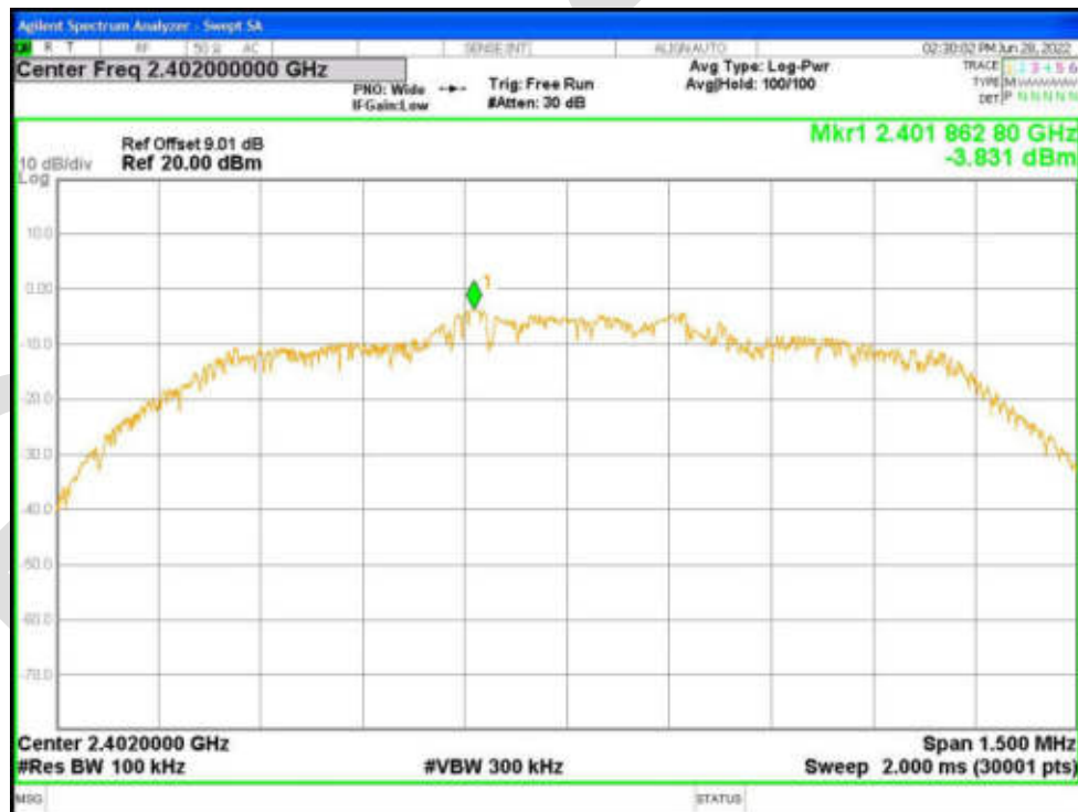
Tx. Spurious NVNT 2-DH1 2402MHz Ant1 Emission
