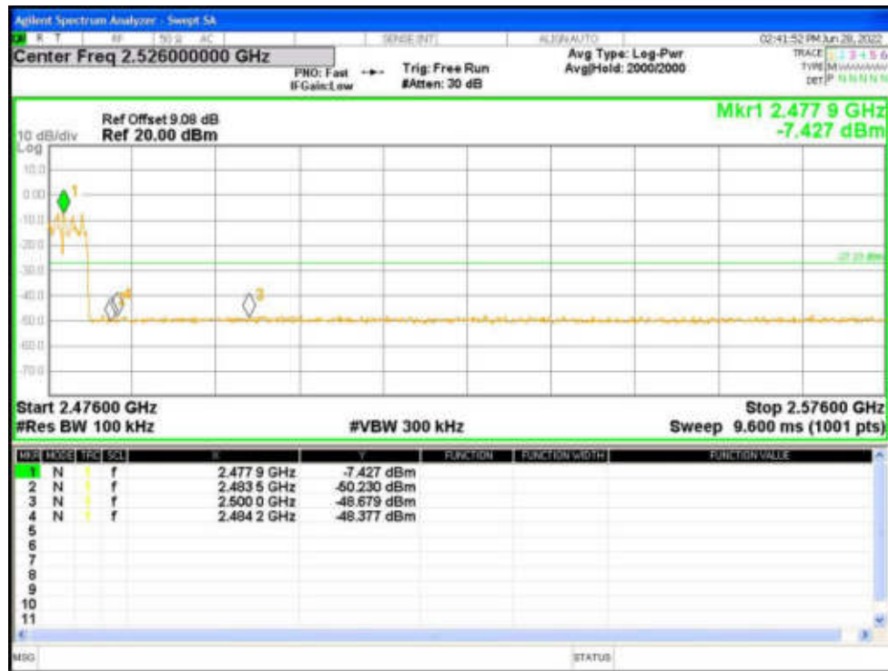
Band Edge(Hopping) NVNT 3-DH1 2402MHz Ant1 Hopping Ref
