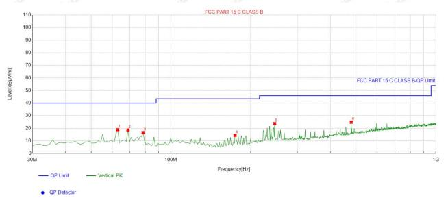
Suspected List Freq. Factor Reading Level Limit Margin Height Angle NO. Polarity [MHz] [dB] [dBµV/m]  $[dB\mu V/m]$ [dBµV/m] [dB] [cm] [°] 63.013013 -14.38 33.28 18.90 40.00 21.10 100 229 Vertical 68.838839 -15.56 21.35 234 Vertical 34.21 18.65 40.00 100 78.548549 308 -17.29 33.92 16.63 40.00 23.37 100 Vertical 4 174.67467 -16.88 31.28 14.40 43.50 29.10 100 0 Vertical 5 246.52652 -13.2336.97 23.74 46.00 22.26 100 27 Vertical 479.55956 -7.79 32.68 24.89 46.00 21.11 100 128 Vertical
