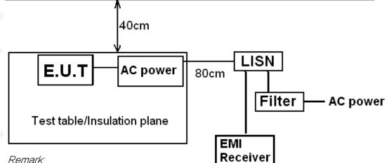
Remark: E.U.T: Equipment Under Test LISN: Line Impedence Stabilization Network Test table height=0.1m
