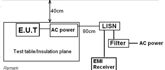
E.U.T: Equipment Under Test LISN: Line Impedence Stabilization Network Test table height=0.1m
